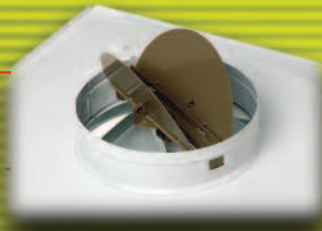
Diffusers feature a long 2 1/4" collar with a form rib for easy flex duct connection and slots for quick attachment of Butterfly Damper.
